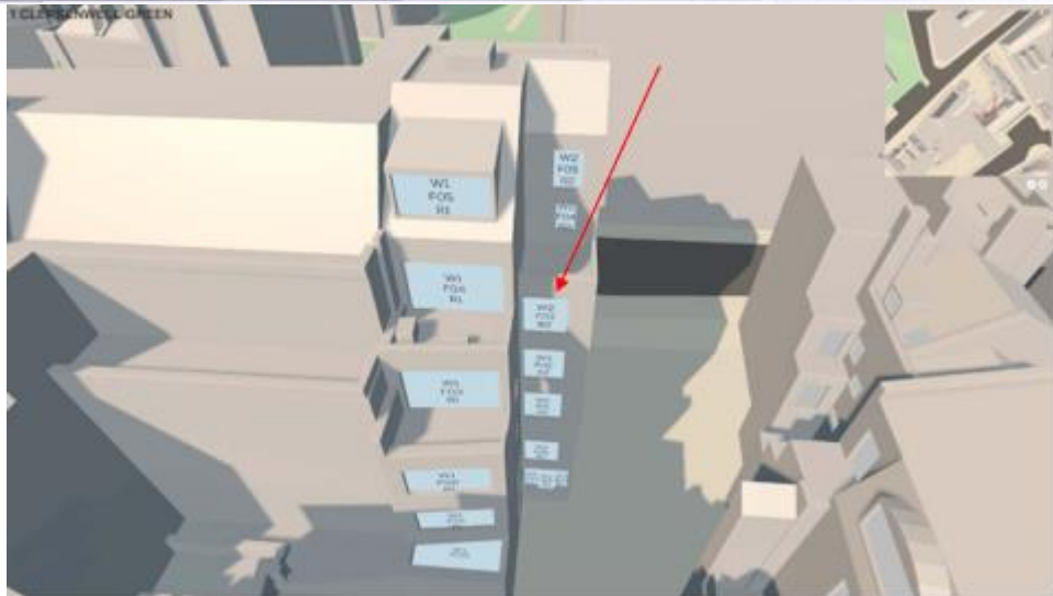
Image 22 & 23: Rear elevation and windows affected assessed under BRE guidance (all now passing)
